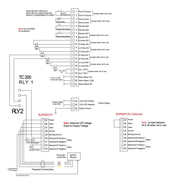
Note: If remote mounting of ignition module is preferred, the ACL 5000R remote mount kit is available upon request
