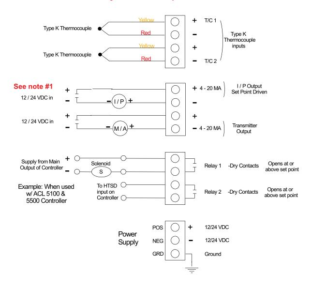
Note #1 4-20mA (1) may be programmed to provide 4-20mA from setpoint. See 4-20mA output specifications.
