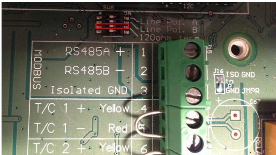
Figure 3 - 120 ohm Termination Resistor DIP Switch
