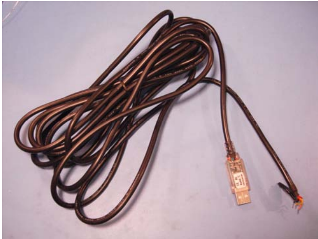
Figure 10 - FTDI Chip USB-RS485-WE-5000-BT, 5m, USB to RS-485 Cable
